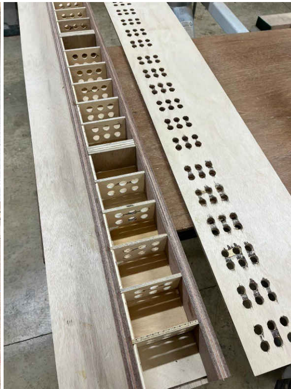
Figure 2.7: Caisson elbow connection(left) and internal screens chambers (right)
