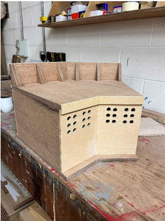
Figure 2.7: Caisson elbow connection(left) and internal screens chambers (right)
