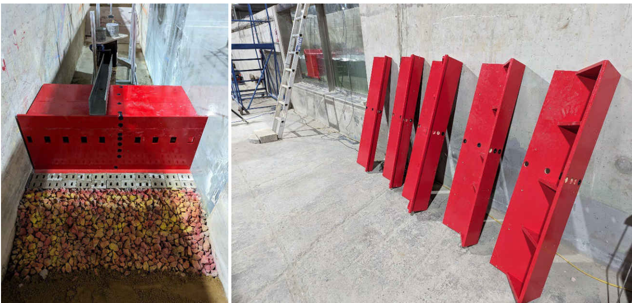
Figure 2.5: Model caisson; wall design 1 (left) and 5 alternatives (right)
