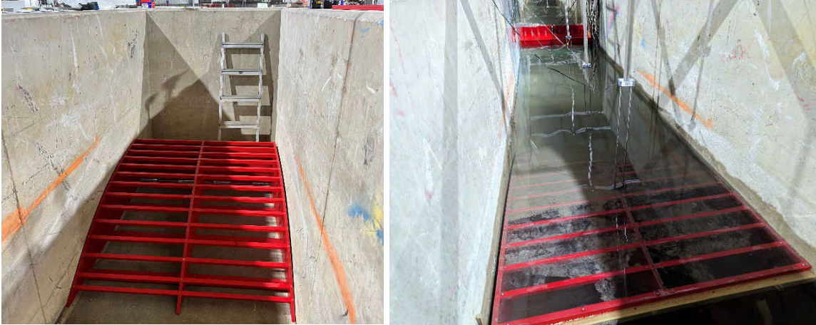
Figure 4.2: Absorption parabolic beach at end of flume to limit reflections and control SWL
