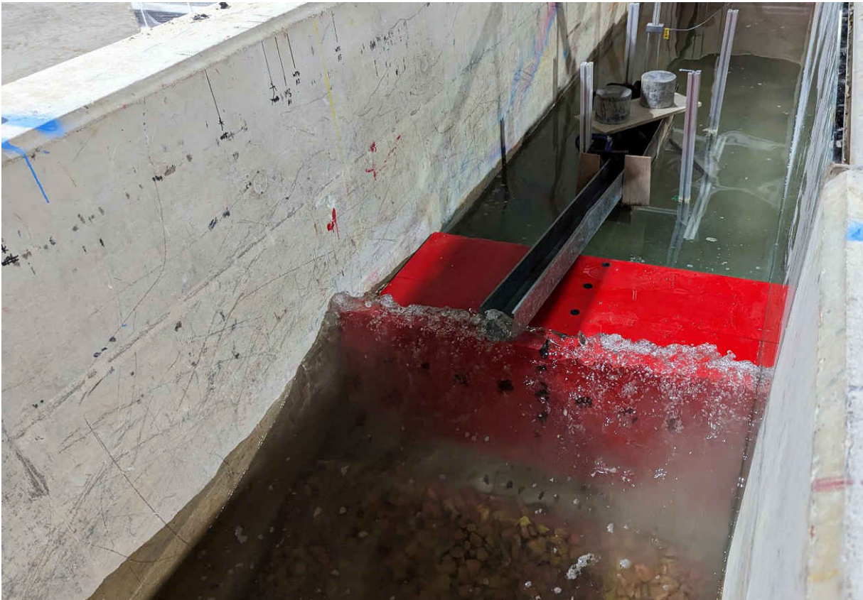
Figure 2.6: Overtopping shoot and tank behind caisson breakwater
