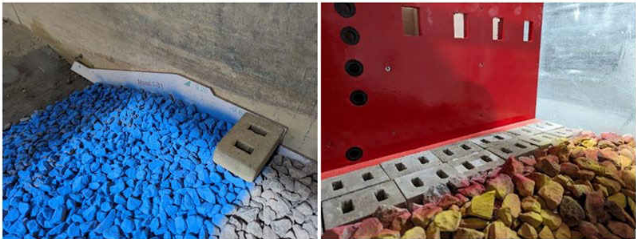
Figure 3.3: Caisson toe blocks
