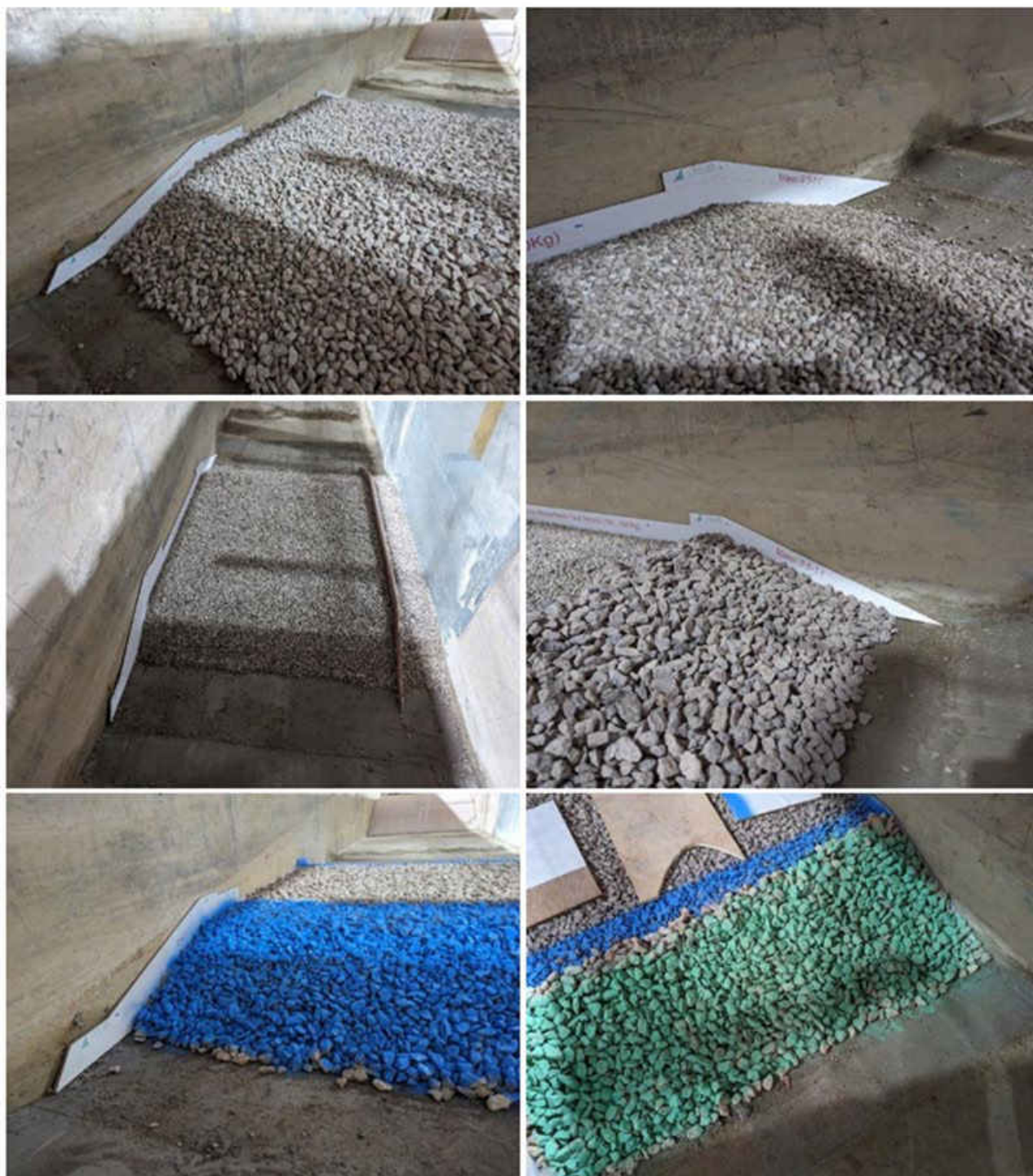
Figure 3.2: Breakwater mound construction sequence
