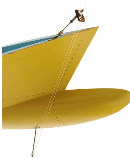
Relative single resistance wave height probe (mounted at ship model)
