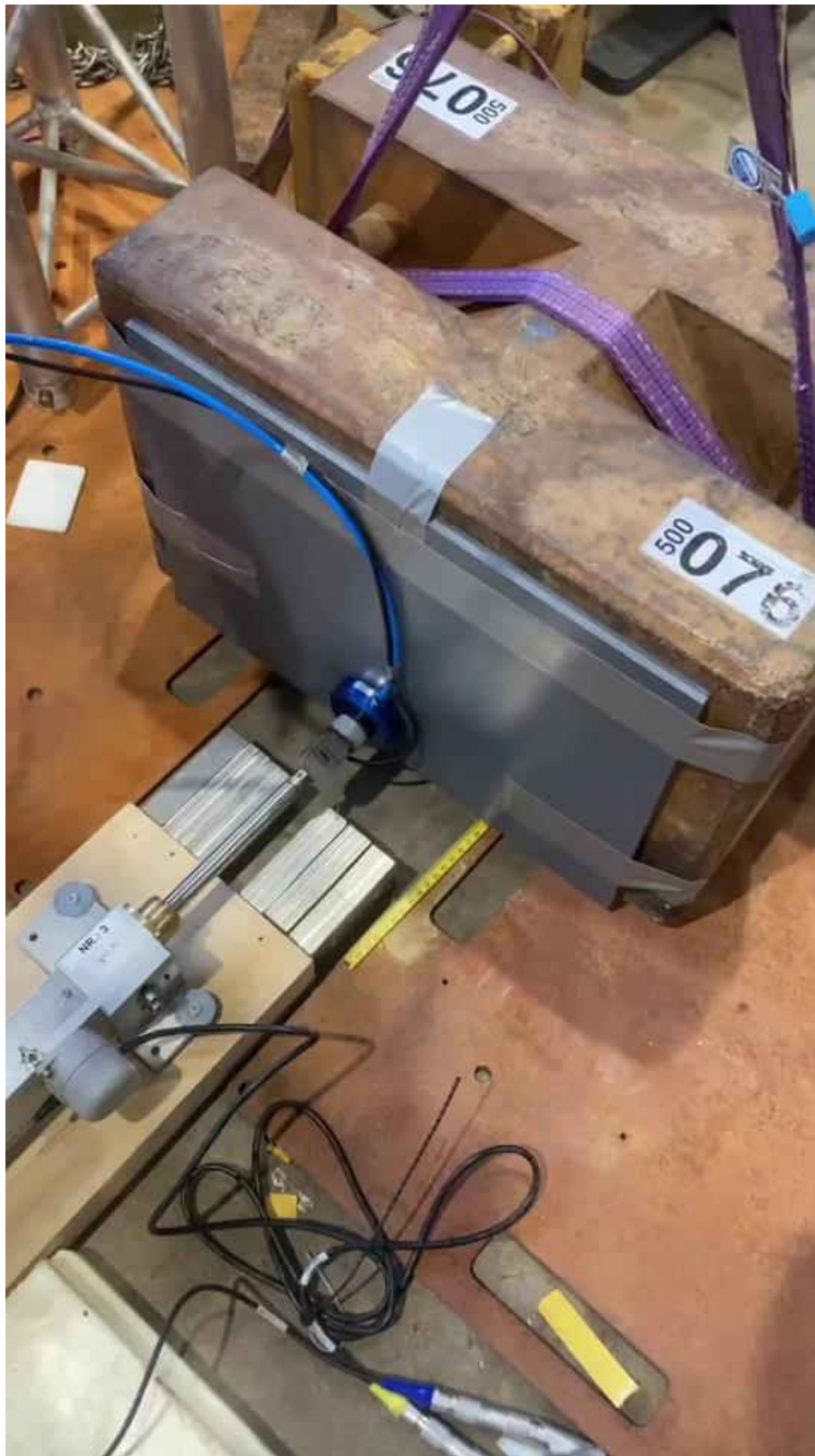
PHOTO 23 JETTY FENDER ACTUATOR DURING CALIBRATION
