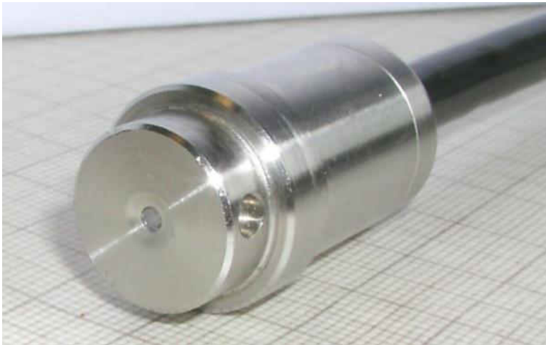
The pressure sensor showing the active measuring area in the centre of the flush diaphragm
