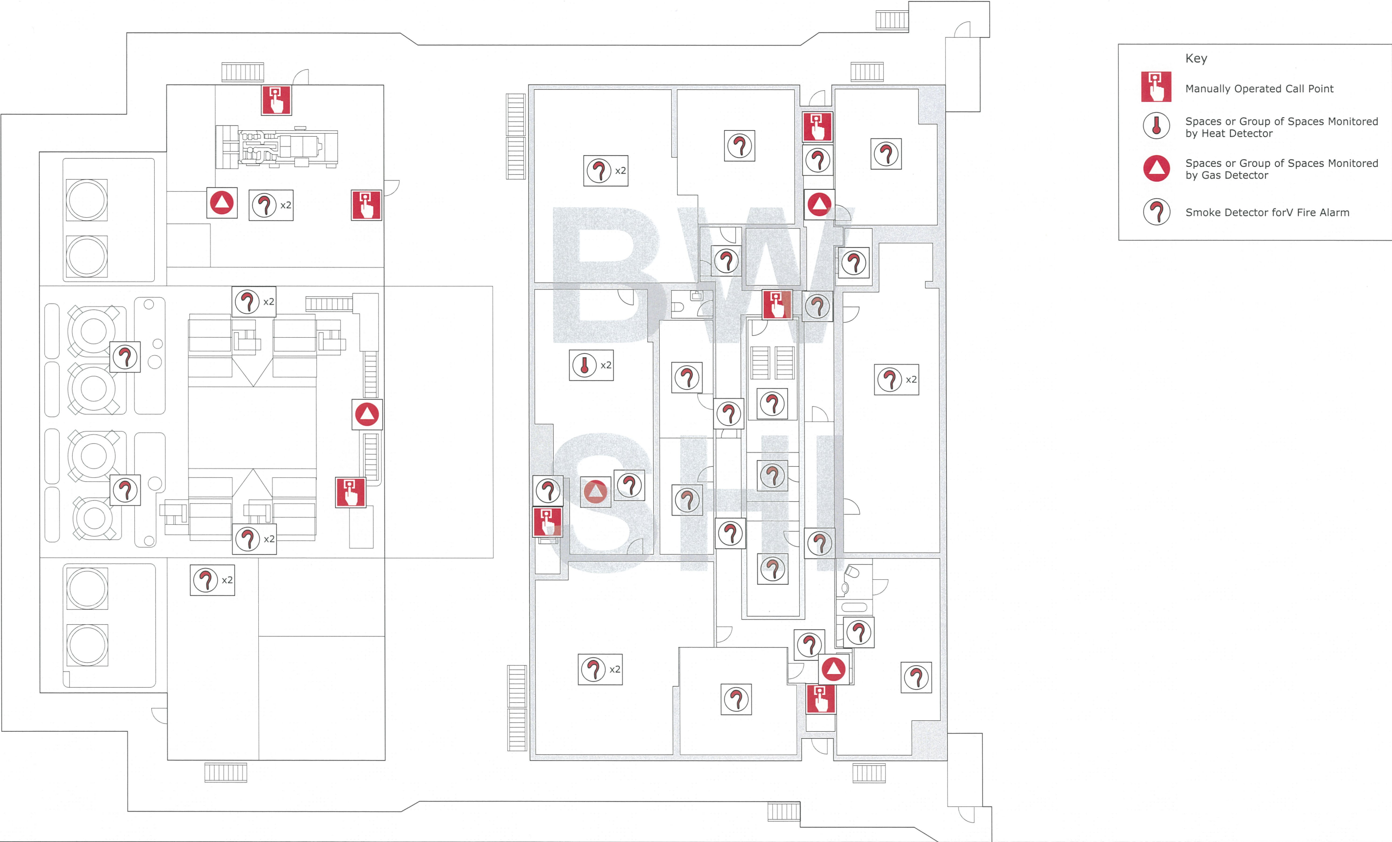
Illustration 8.9i Fire Detection and Alarm Equipment - A Deck
