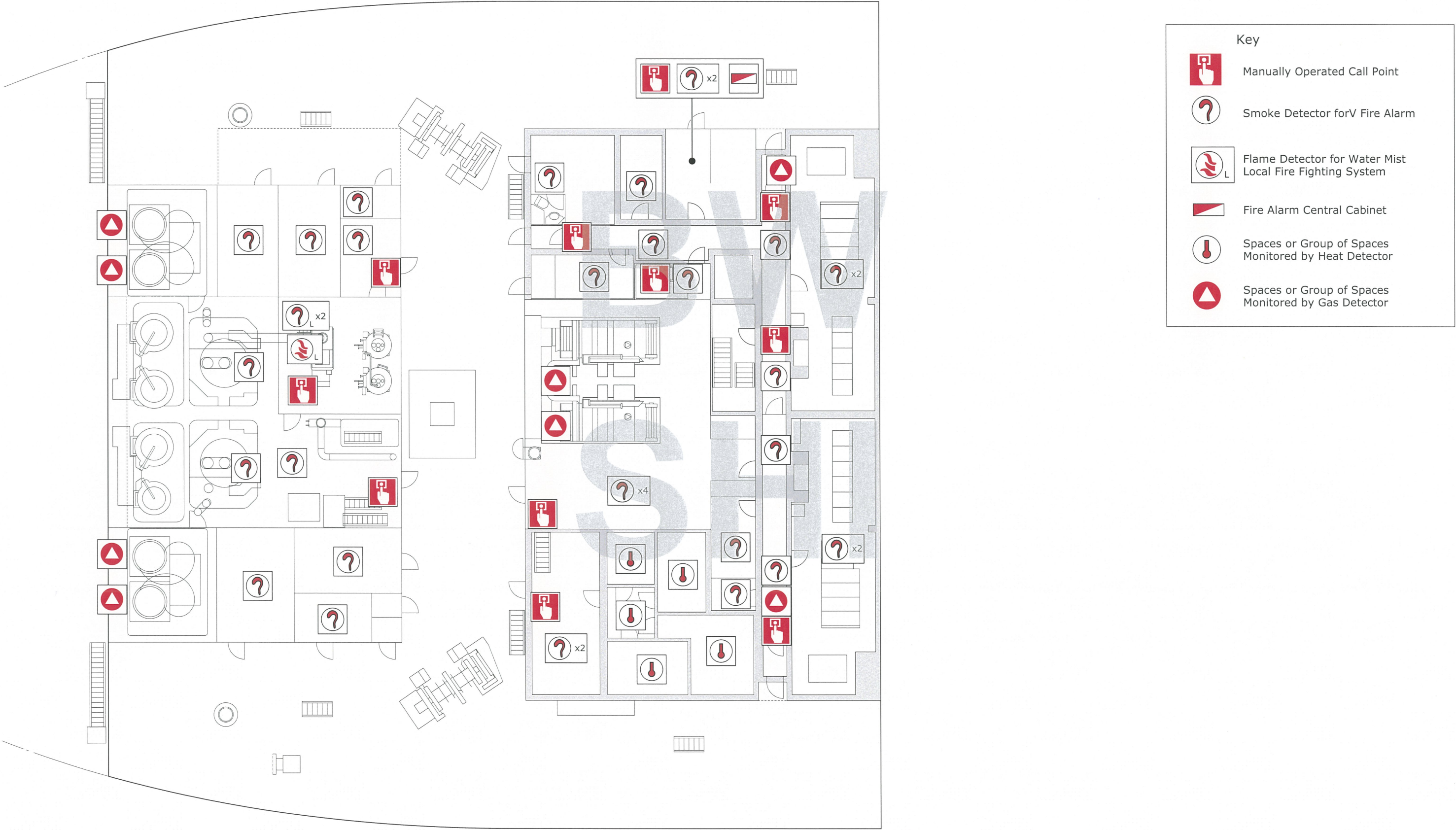
Illustration 8.9g Fire Detection and Alarm Equipment - Accommodation Upper Deck
