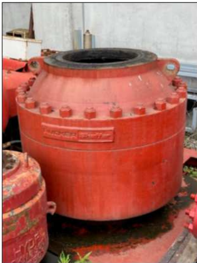
Figura 4.1.3 – Diverter Shaffer 21 1/4"
