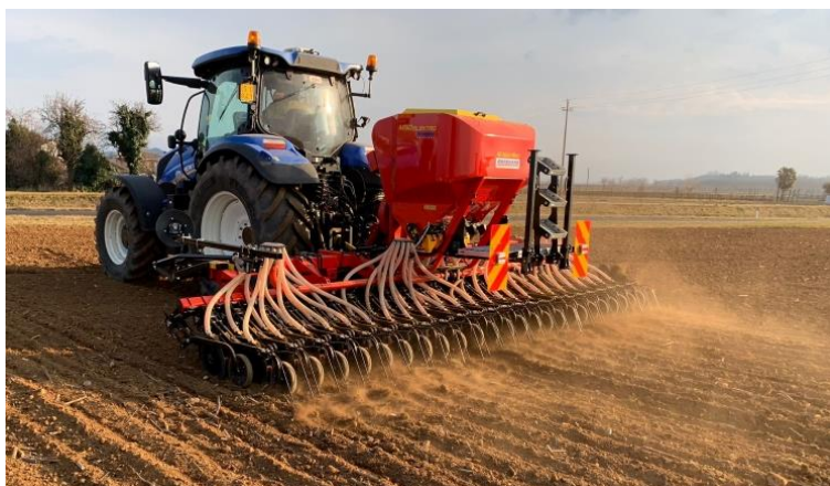
Figura 31 – Seminatrice a file interrate universale
