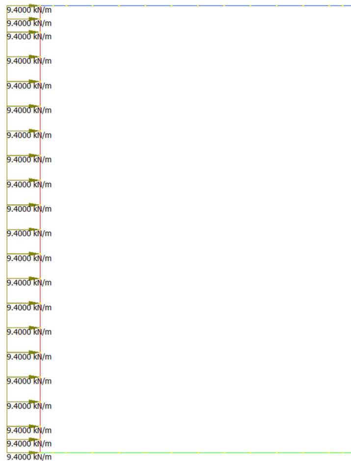
Figure 8-10: Carico stradale SN
