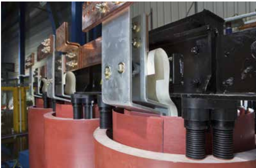
HV coil support wedges
