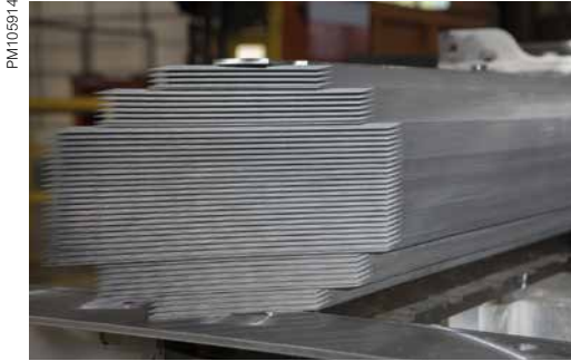
Magnetic core being assembled
