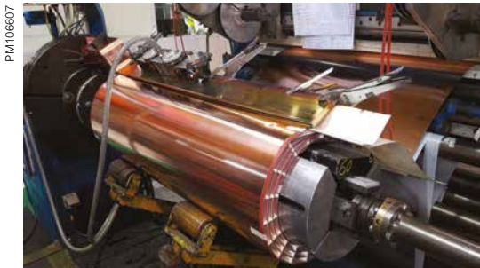
LV winding with foil technology
