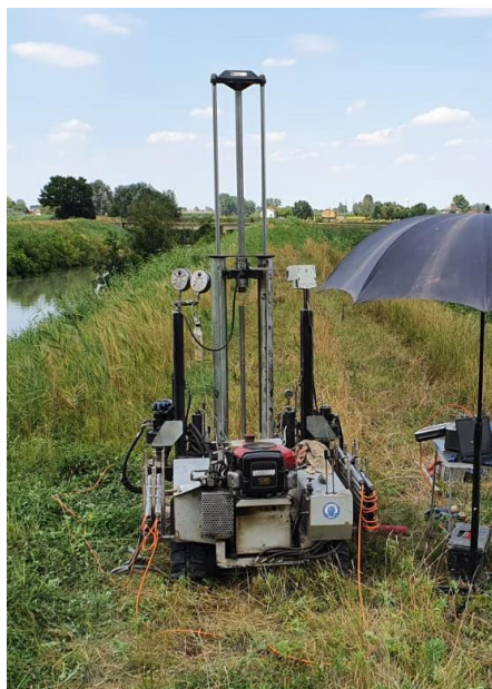
Fig. 3.2 – Penetrometro Deep Drill SP200
